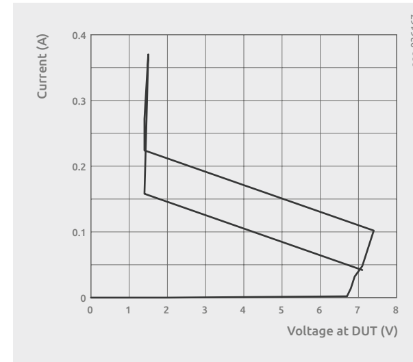
Figure 13 | I-V-hysteresis curve of a Treos ESD protection device. 5 MHz test signal with 50% duty cycle and 50 \Omega output resistance of the signal generator
