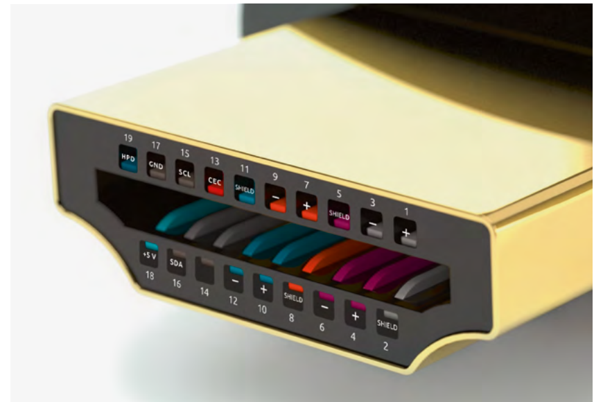
Figure 31 | Pinout and front view of an HDMI type-A plug
