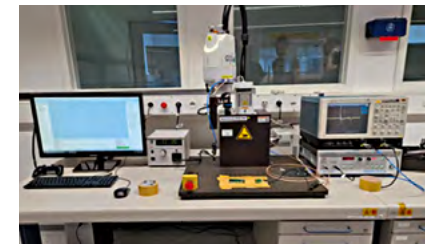
Figure 27 | EMI scanner for time domain ESD analysis.
