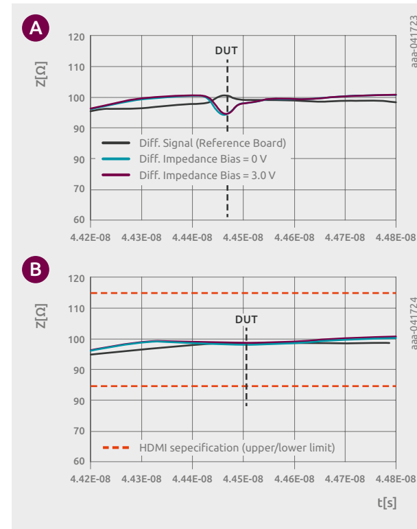
Figure 23 A and B | Impedance curve of an ESD diode on a differential line pair with Z_0 = 100 Ω, measured with t_{rise} = 40 ps and t_{rise} = 200 ps compared to reference.
