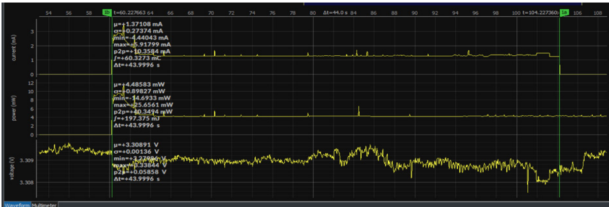
Figure 3: MCU current consumption for one cycle of active operation (1.37 mA of average current).
