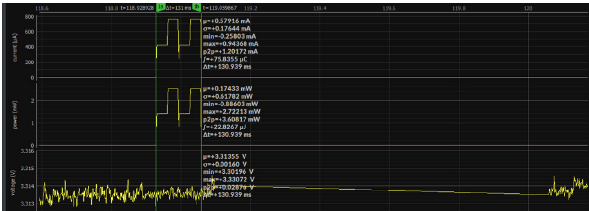
Figure 5: BME680 Sensor Current Profile.
