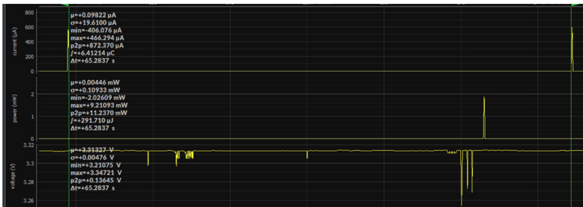
Figure 6: BME680 Sensor Sleep Mode current profile (0.098 \mu\text{A} of leakage current).
