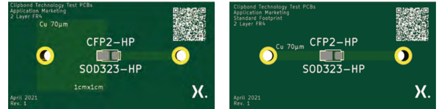
Figure 51 | Example CFP2-HP test boards: 1cm² mounting pad for cathode vs. standard footprint.
