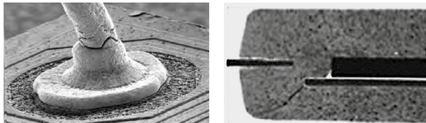
Figure 97 | Potential failure modes might be caused by manufacturing: broken wedge (left), package crack.
